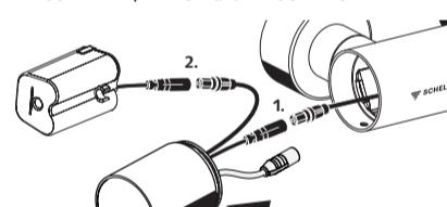
Bluetooth® module VITUS for use with: VITUS VW-E-T, VW-C-T and VITUS VD-C-T with solenoid valve for thermal disinfection
