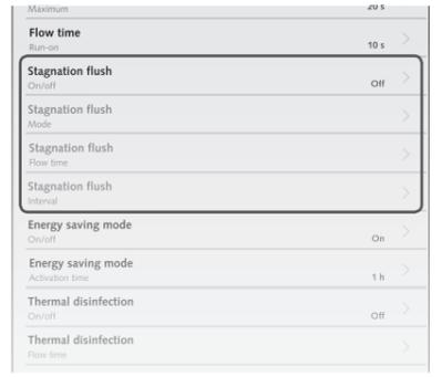
The configuration options for the stagnation flush described here are related only to the fitting and not to the stagnation flush configurable under "Hygiene".
