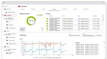
Information about hygiene flushes and temperature curves help operators to analyse their system(s) accurately:
