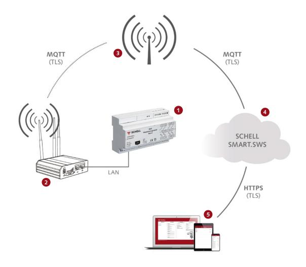
From a server-level view to a general overview of all of the buildings: messages, calculated water consumption and much more is all attractively visualised by the SMART.SWS dashboard. The views vary by user role, so as to ensure that only the relevant data is displayed for the individual currently logged in.
