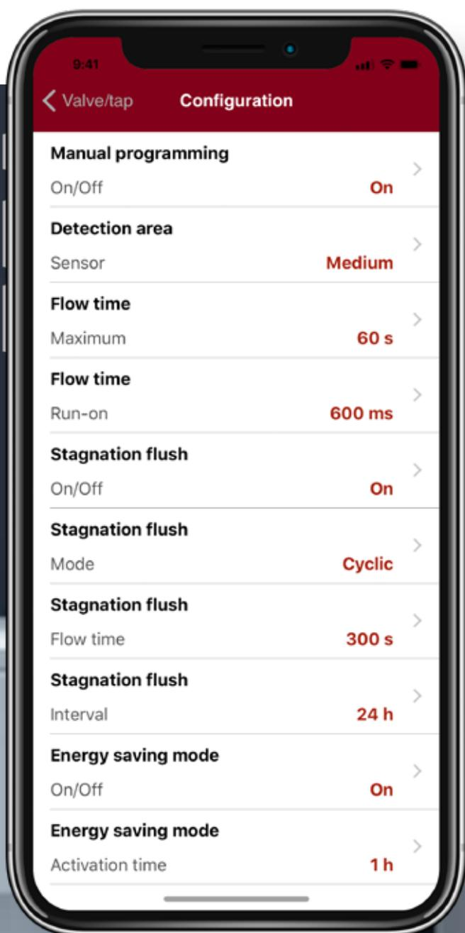
Simply insert the SSC Bluetooth® module between the tap and the power supply, and then configure the tap with the user-friendly smartphone app. To finish up, simply remove the SSC Bluetooth® module again.
