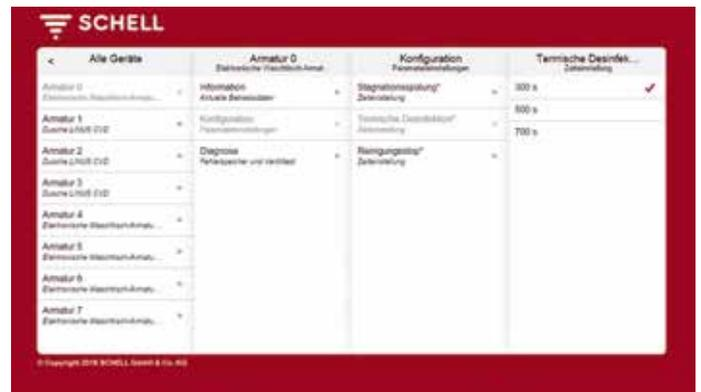
To provide end-to-end documentation that TD has been performed properly, a temperature sensor can be integrated that scans and records the water temperatures. All flushing runs can be programmed individually, logged on the micro SD card integrated into SWS server and repeated at any time.
