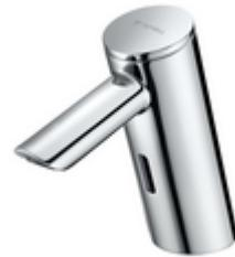
Contactless, sensor-controlled tap with innovative ToF technology. Insensitive against reflective materials such as mirrors, safety vests, etc. With integrated Bluetooth® interface. Configurable via SCHELL app. Suitable for networking with the SCHELL SWS water management system. Battery operation. With extended outlet 134 mm.
